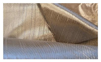
ISOMATEX's **non crimped (NCF) Quadriaxial fabric** is made out of 4 layers of unidirectionally placed FILAVA<sup>™</sup> direct rovings oriented at 0°, -45°, 90° and +45° respectively. The layers then are stitched together by a polyester yarn, rather than woven, so there is no crimp in the rovings according to the sketch below.
